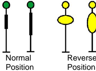
Note: Switch targets may be different shapes than illustrated but must not be diamond shape.
