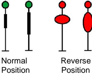
Note: Switch targets may be different shapes than illustrated but must not be diamond shape.
